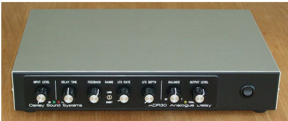
The ADR30 built into a Takachi YM300 case with Schaeffer engraved panel overlay.
