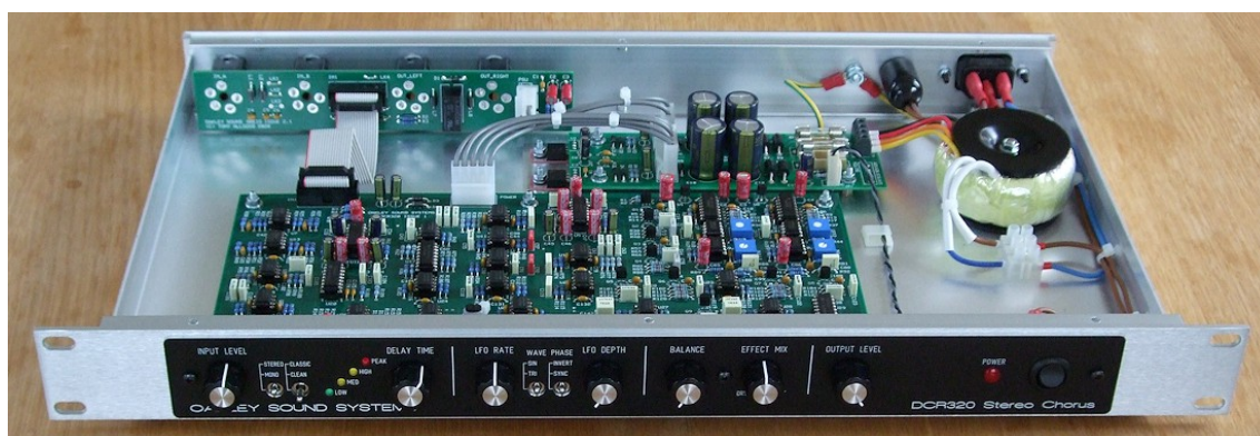
The first prototype unit built into a Bryant Broadcast 1U 250mm deep 19" rack enclosure with the Schaeffer front overlay panel attached. This one has an internal toroidal mains transformer.
