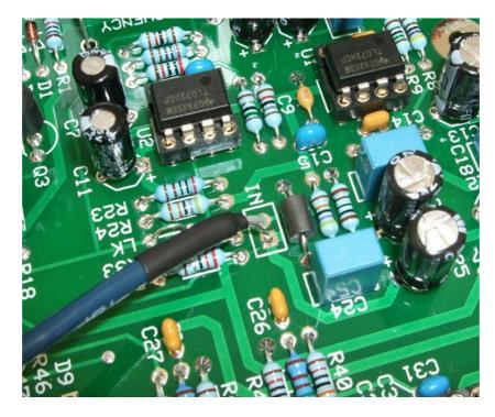
The top end of the screened cable. The screen being connected to pin 1 and the core of the cable connected to pin 2. Here I have used a bit of black heatshrink to keep things neat and tidy.
