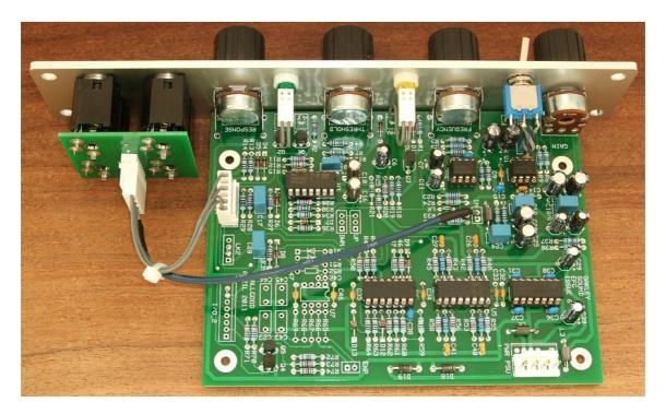
*This is the prototype of the issue 6 standard EFG module behind a natural finish 1U wide Schaeffer panel. Note the use of the optional Sock4 socket board to facilitate the wiring up of the six sockets.*
