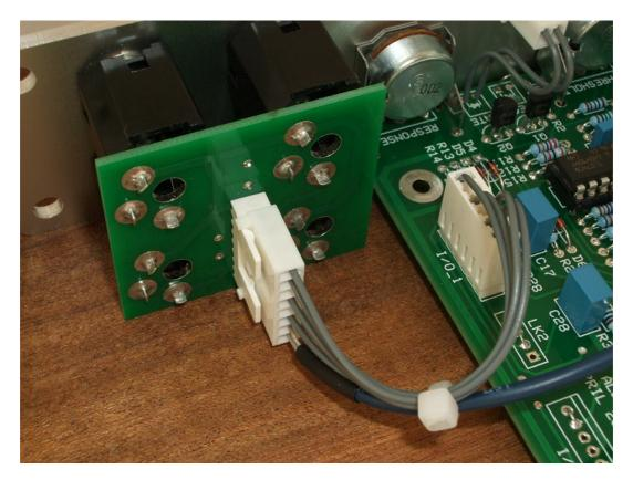
This shows the Sock4 connection on a standard EFG. Here I have used Molex KK 0.1" connectors. These are solderless crimp fixings that make a low cost but effective connection. Pin 7 and 8 of the interconnect are connected via a screen cable (also crimped into the Sock4's Molex housing) and go on to the pre-amp input, IN, on the main board.
