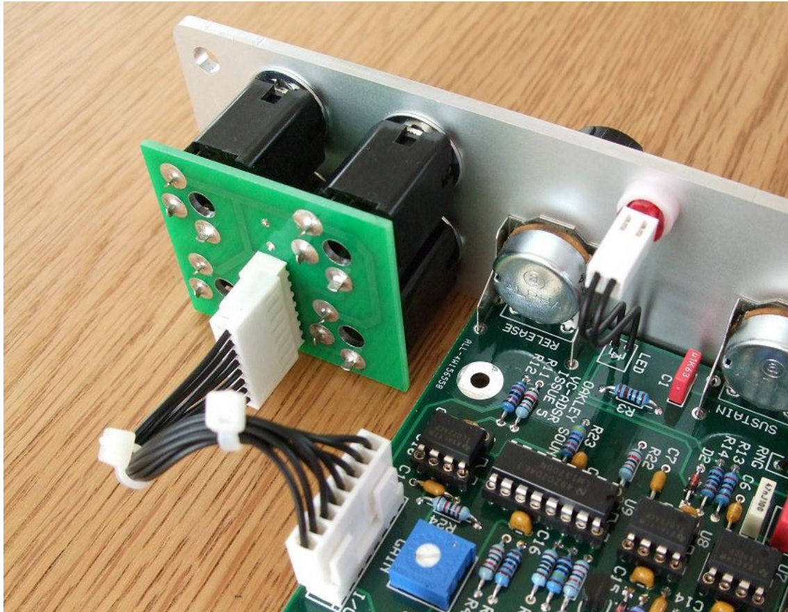
The prototype unit showing the detail of the board to board interconnect. Here I have used the Molex KK 0.1" system to connect the Sock4 to the main PCB.
