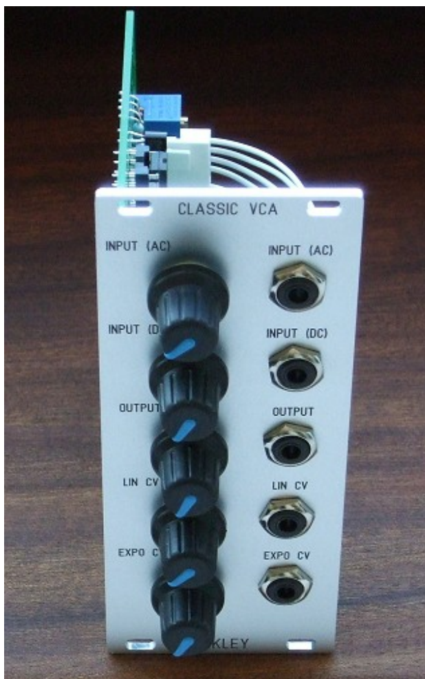
The prototype Classic VCA module using a 10HP wide Schaeffer panel. Note that on this module the sockets are on the right of the pots. The Krisp1 manufactured version has the pots to the left and fitted with an 8HP wide panel. The functionality is the same however.
