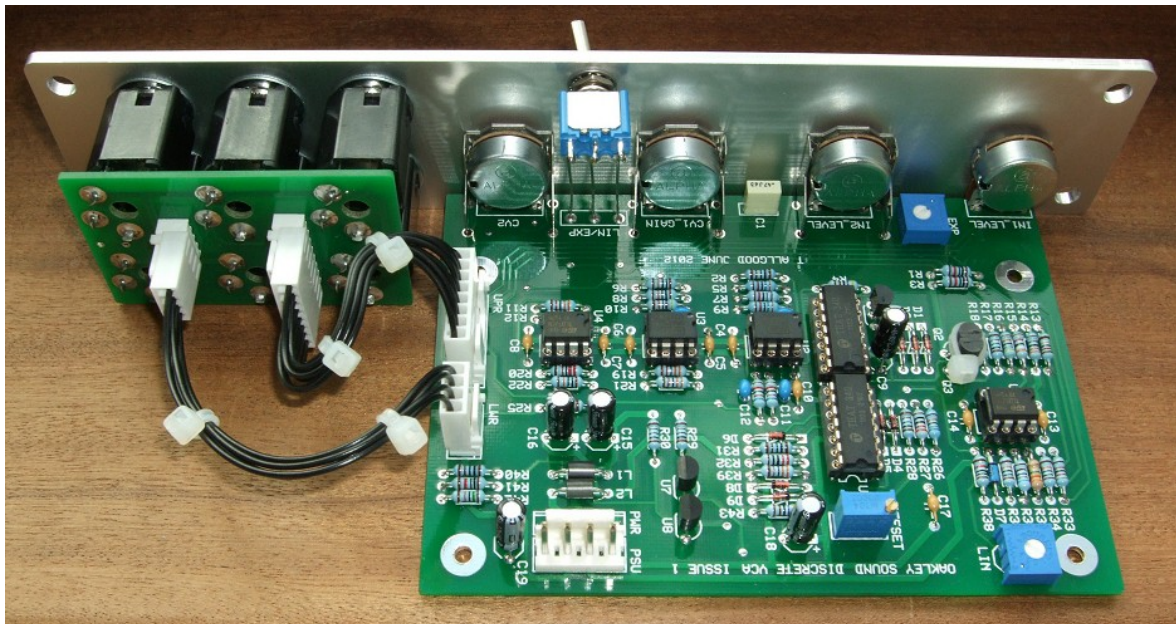
The issue 1 Oakley Classic VCA module behind a natural finish 1U wide Schaeffer panel.
