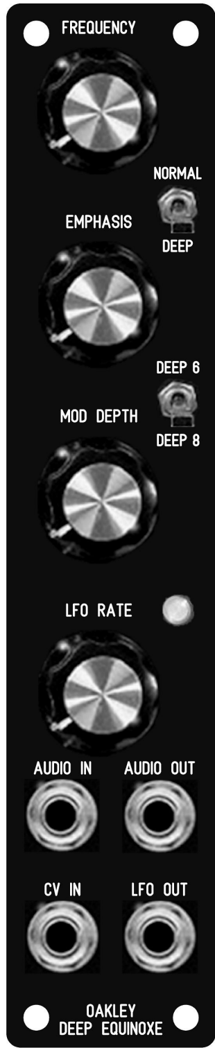
The 1U wide panel design for the two switch variant of the Deep Equinox for MOTM format systems. The fpd file for this panel can be found on the project webpage.
