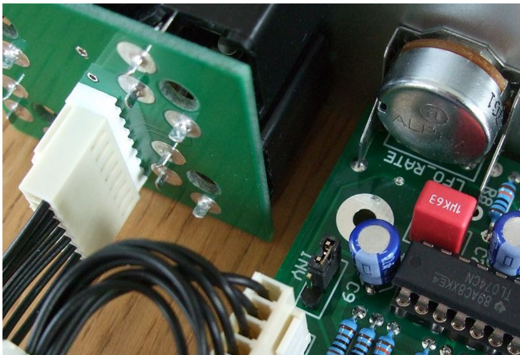
Here we can see the three pin header and two way jumper that selects the LFO mode. In the position shown in the photograph the LFO OUT will produce an inverted signal - the jumper is aligned with the letters INV on the circuit board.
