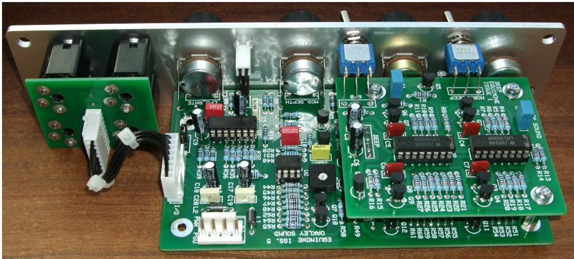
The prototype Oakley Deep Equinoxe module behind a natural finish Schaeffer panel. The Deep Equinoxe board is the smaller one mounted above the standard Equinoxe PCB.
