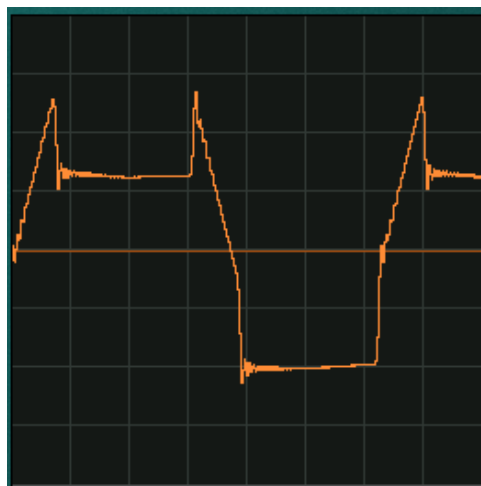
Figure 6. Track mode showing a negative offset voltage making both replacement voltages move downwards.
