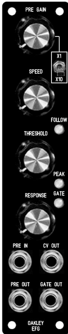
The suggested front panel design for the standard EFG in a single width MOTM format.
