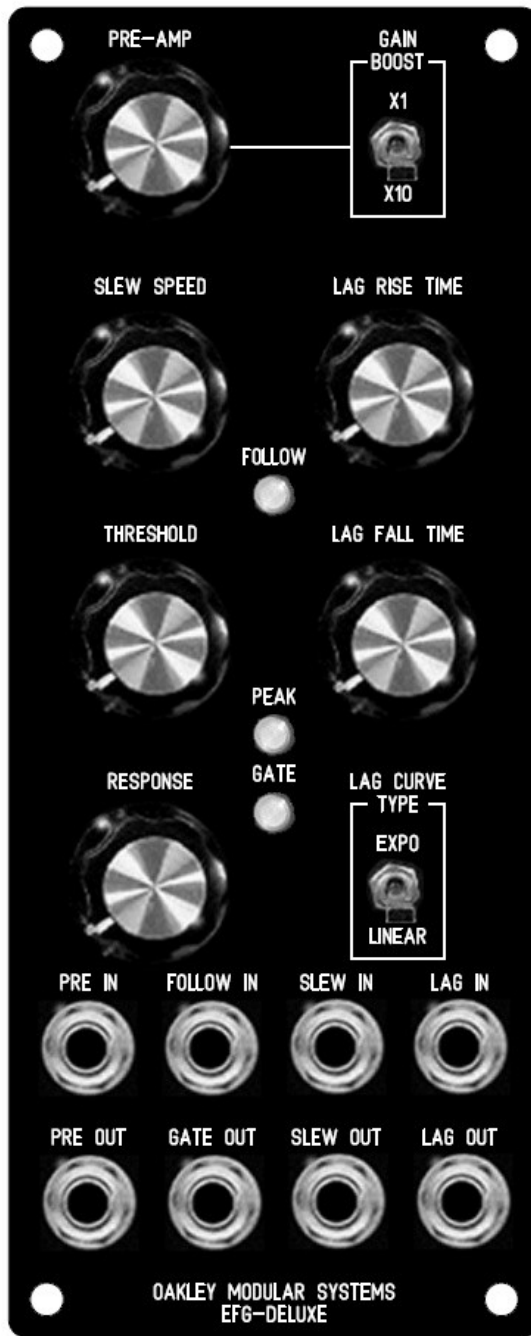
The suggested panel design for the EFG-Deluxe module in the 2U wide MOTM format
