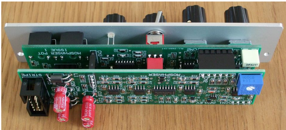
The module comprises of two circuit boards connected together with three six way and one eight way 0.1" SIL headers and sockets.
