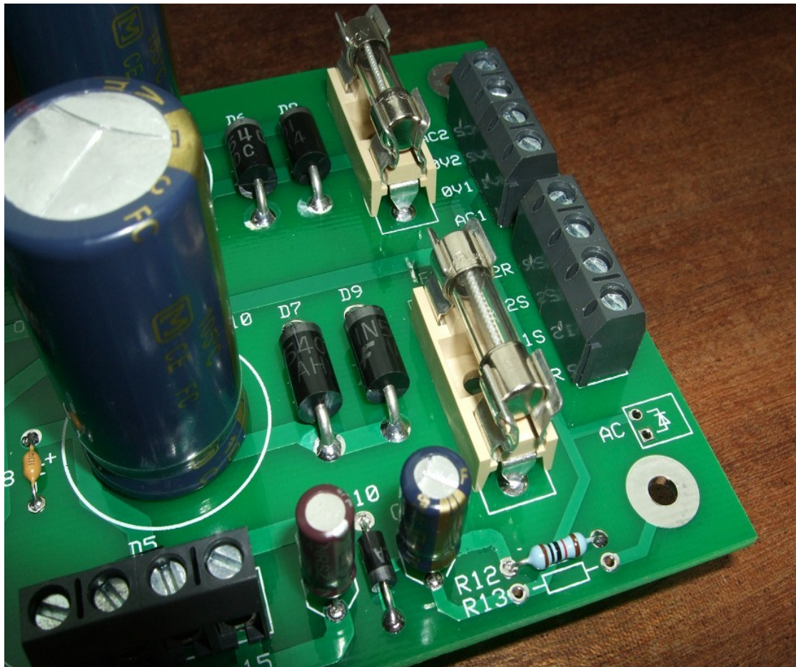
This shows the two fuse holders fitted to the prototype board. R13 is not fitted on this particular build but it would normally be a wire link.
