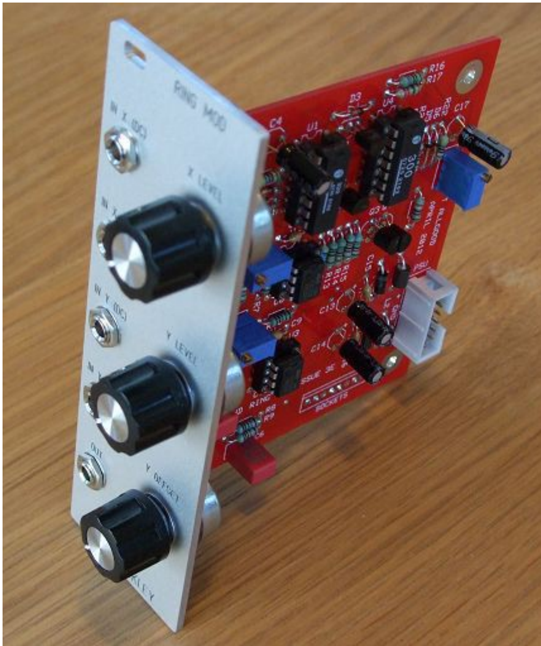
The prototype 8hp wide Oakley Ring Modulator. The faceplate is a natural finish panel from Scheaffer.
