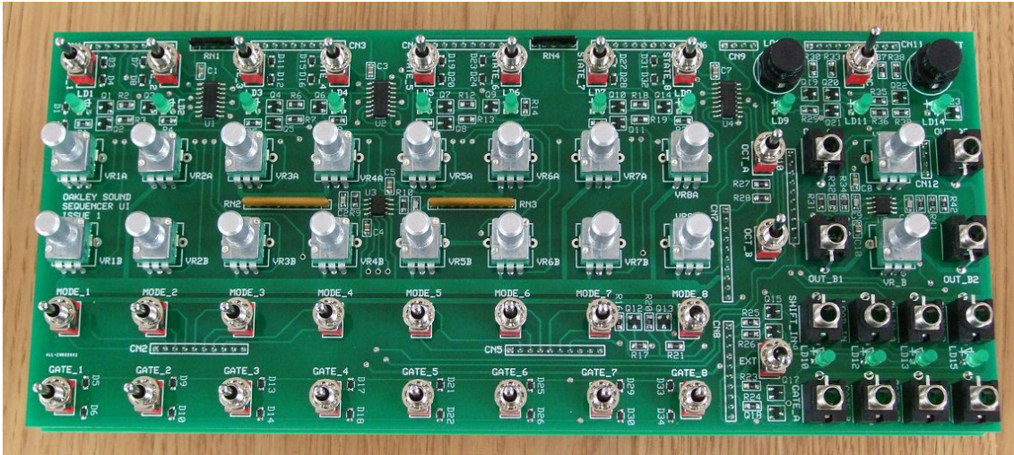
The original issue 1 pot and switch board of the sequencer. Issue 1.1 is similar.
