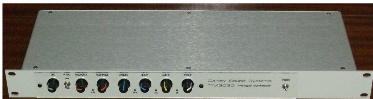
The second issue 1 TM3030 I built. This one has been built into a 19" rack from Holt Broadcast. The front panel legending is achieved with a perspex overlay.
