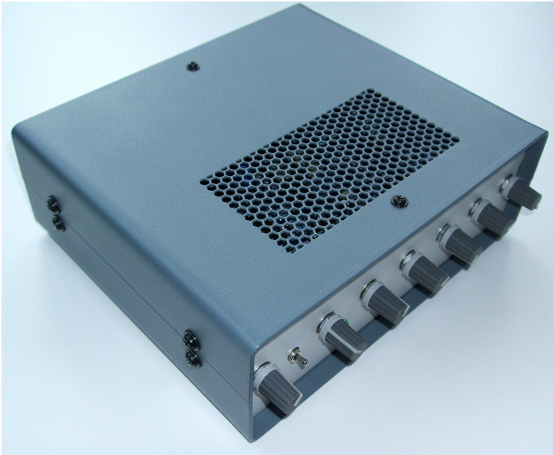
My first issue 2 TM3030 fitted into the three part metal case from RS Components (pt no: 222-020).
