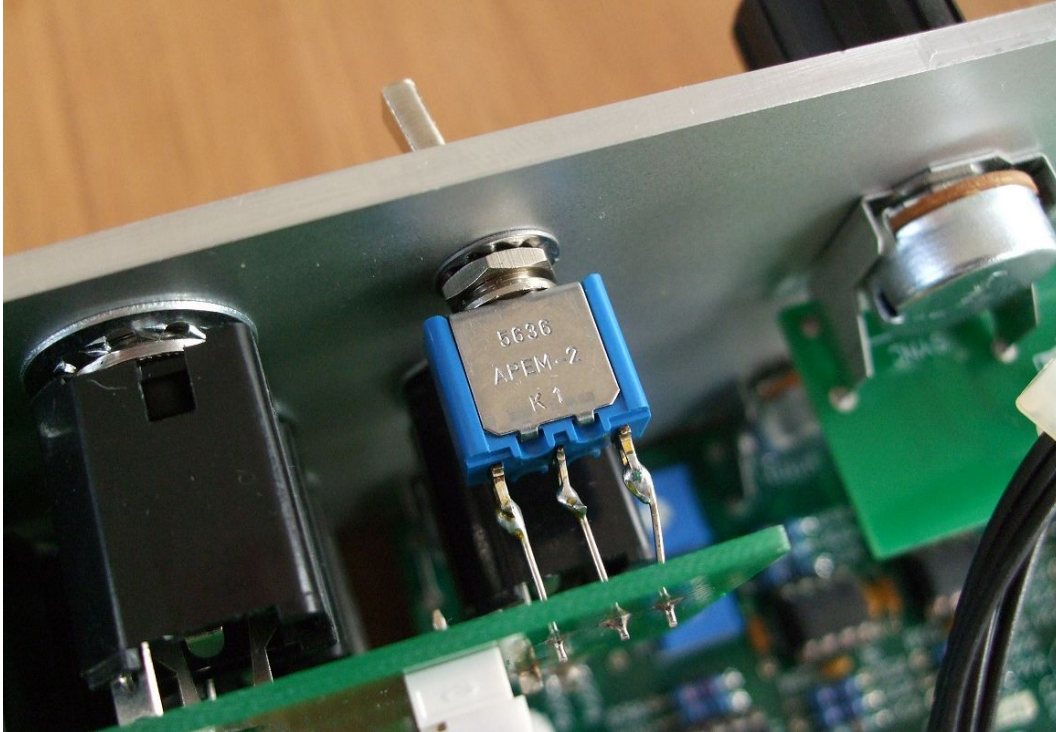
This is an Apem toggle switch mounted to a 3mm Schaeffer panel. Note the spring washer and nut behind the panel.
