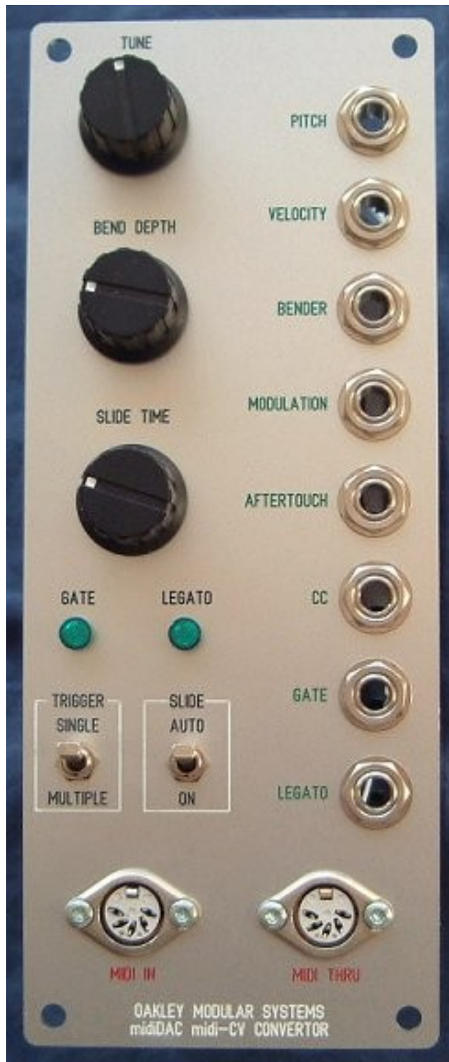
This is the issue 3 midiDAC in a natural finish Schaeffer panel. Note the new rounded corners. The toggle switches are APEM flat blade toggle switches available from Farnell. The round LED holders come from Maplin, whilst the knobs are the Rapid's 'matt black control knobs' for 1/4" fitting.
