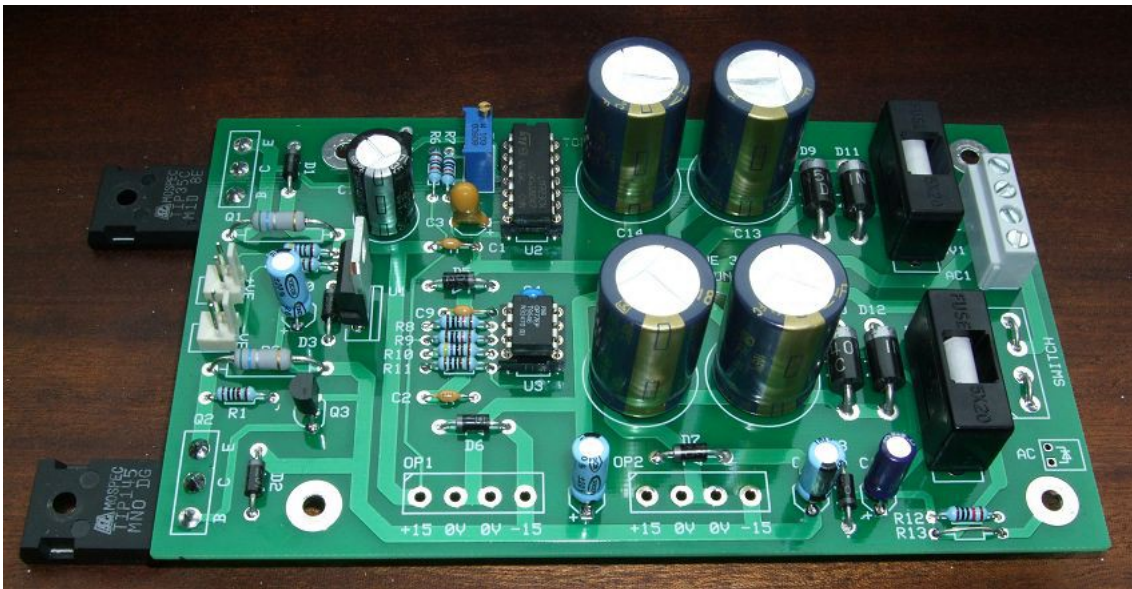
The issue 3 Oakley PSU board awaiting fitting to the front panel.
