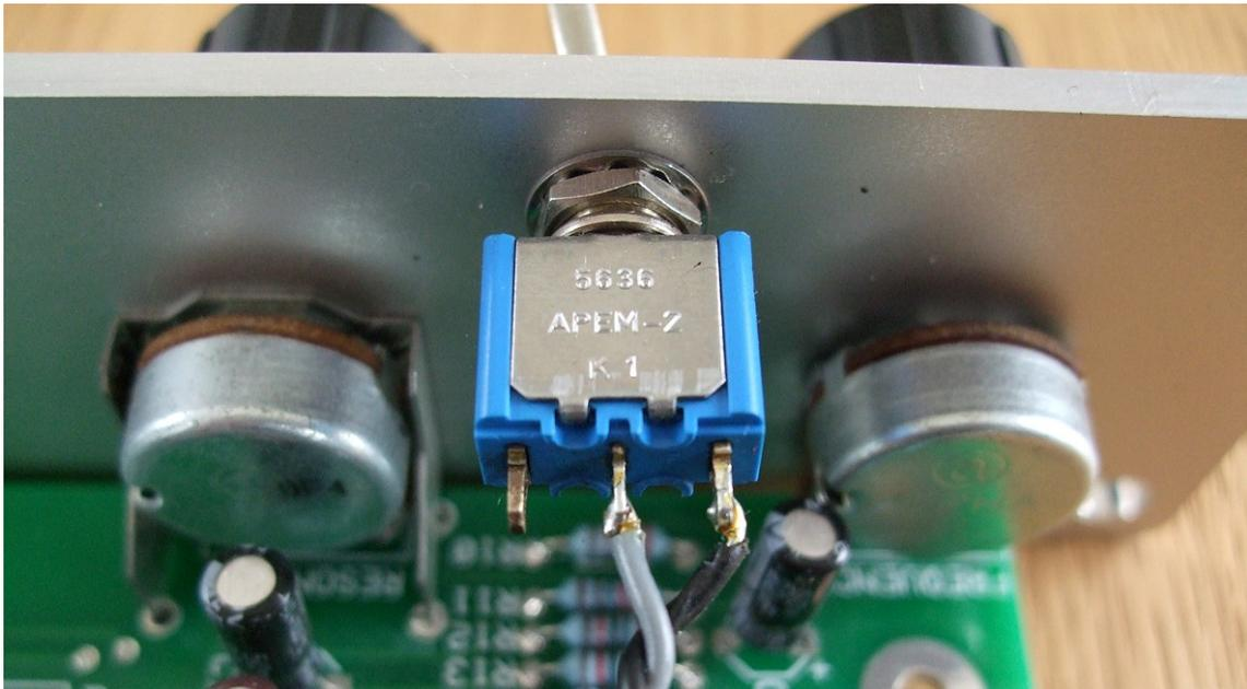
If you are fitting the switch then you need to connect it to the pad marked as SW1 on the Diode Superladder PCB. The switch is wired with a twisted wire pair. This is made by twisting two pieces of insulated multistrand wire together tightly to form a simple cable. You can use two different colours but you don't have to as it does not matter which wire connects to which lug on the switch. Here I have used black and grey wires.
